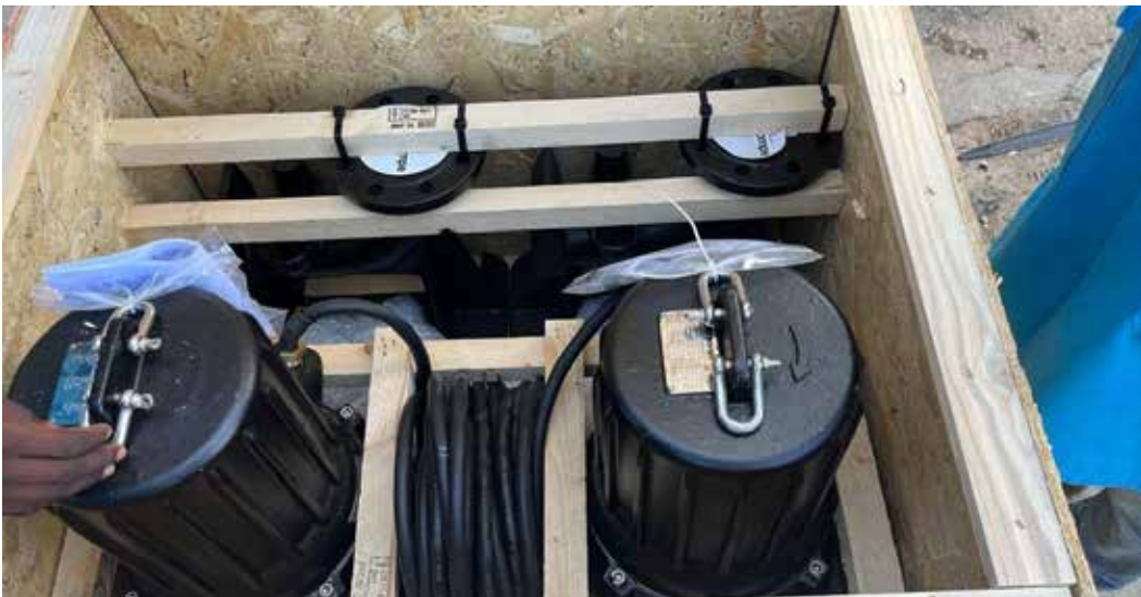
Rovatti Electric submersible pump delivered to site. The pump was submerged in the sump at site
